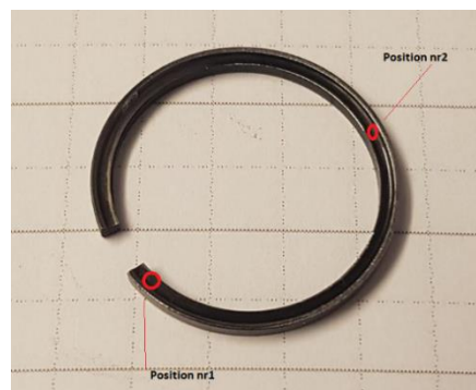
Figure 5. Position 1 and 2 respectively where the sealing ring surface analyses had been done.
