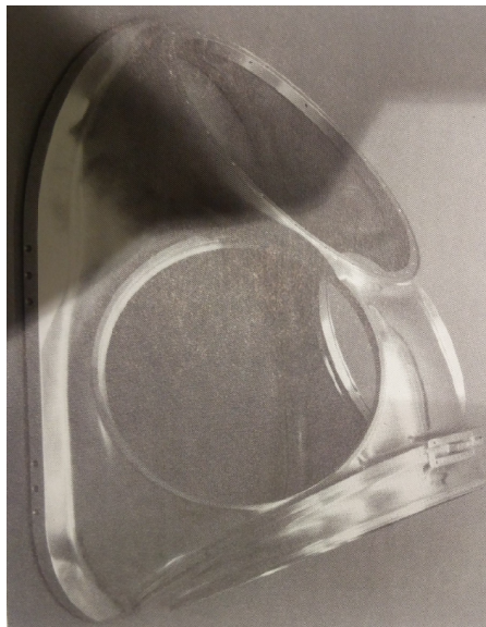
Figure 5.3: ZPS Mark III hard torso shell (left) and Rear entry closure (right)
