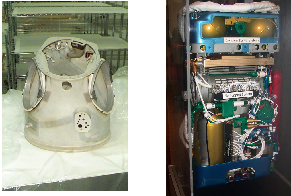
Figure 1.5: HUT and PLSS developed by NASA
