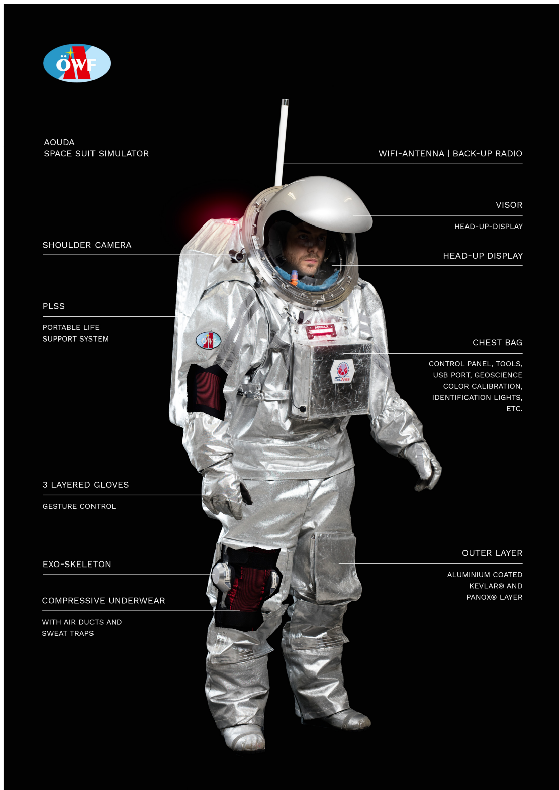
Figure 1.7: Aouda.X Spacesuit and its major components
