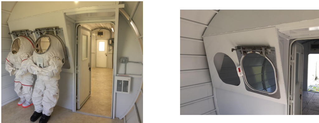
Figure 5.20: NDX Suitport configuration
