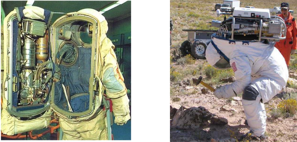
Figure 5.19: PLSS configuration of the Orlan ( left ) and I-suit ( right )
