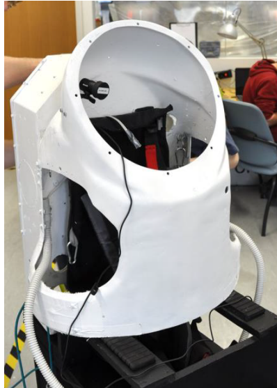
Figure 3.1: Empty HUT (configuration early 2014, here without aluminium reinforcements on the shoulders)
