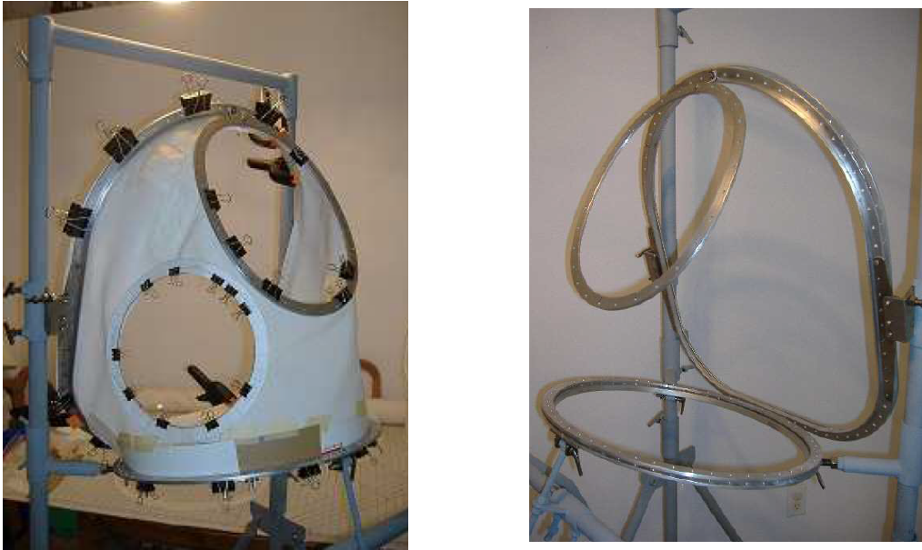
Figure 5.4: NDX-2 HUT ( left ) and Helmet, Rear and Waist rings ( right )
