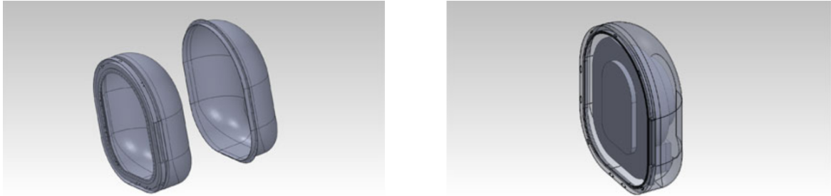
Figure 4.4: Left: Suitport assembly that connects to the NDX-2 and Rover mount and Suitport dock. Right: Dome section of the space suit portion of the Suitport showing a mock up of the PLSS fitting.
