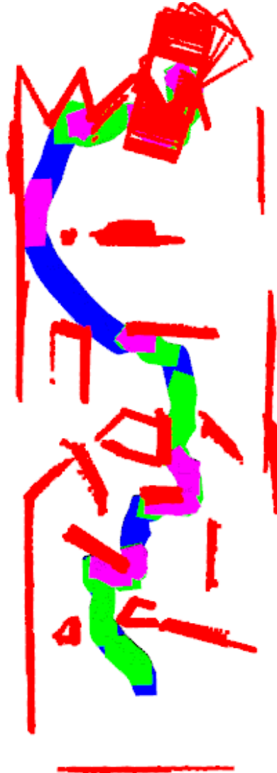
Figure A.51: The path for operator 5 with configuration 2 in the user study. Red is obstacles detected by sensor, blue is the UAV, green is when haptic feedback is activated, and pink indicates collision.
