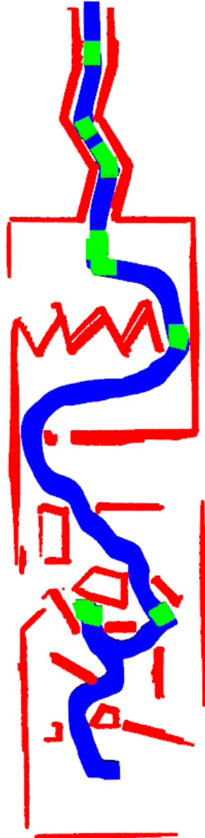
Figure A.9: The path for operator 1 with configuration 5 in the user study. Red is obstacles detected by sensor, blue is the UAV, and green is when haptic feedback is activated.
