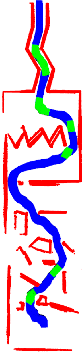
Figure A.33: The path for operator 3 with configuration 5 in the user study. Red is obstacles detected by sensor, blue is the UAV, and green is when haptic feedback is activated.
