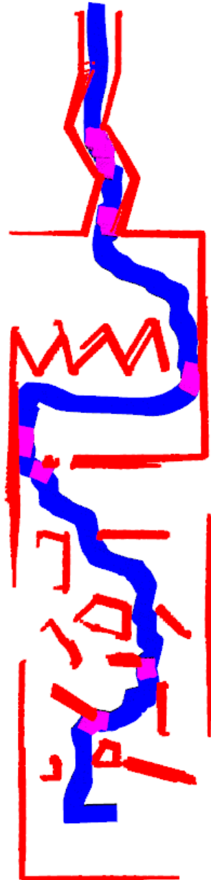
Figure A.7: The path for operator 1 with configuration 4 in the user study. Red is obstacles detected by sensor, blue is the UAV, and pink indicates collision.
