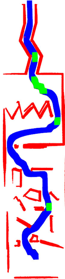
Figure A.93: The path for operator 8 with configuration 5 in the user study. Red is obstacles detected by sensor, blue is the UAV, and green is when haptic feedback is activated.
