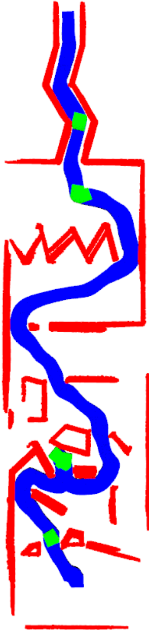
Figure A.21: The path for operator 2 with configuration 5 in the user study. Red is obstacles detected by sensor, blue is the UAV, and green is when haptic feedback is activated.
