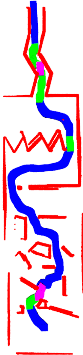
Figure A.95: The path for operator 8 with configuration 6 in the user study. Red is obstacles detected by sensor, blue is the UAV, green is when haptic feedback is activated, and pink indicates collision.
