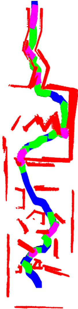
Figure A.59: The path for operator 5 with configuration 6 in the user study. Red is obstacles detected by sensor, blue is the UAV, green is when haptic feedback is activated, and pink indicates collision.
