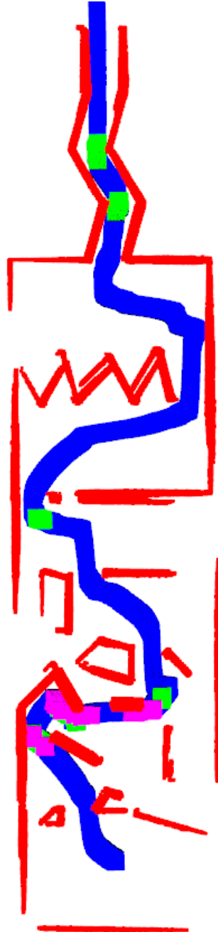
Figure A.3: The path for operator 1 with configuration 2 in the user study. Red is obstacles detected by sensor, blue is the UAV, green is when haptic feedback is activated, and pink indicates collision.
