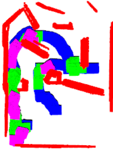
Figure A.27: The path for operator 3 with configuration 2 in the user study. Red is obstacles detected by sensor, blue is the UAV, green is when haptic feedback is activated, and pink indicates collision.
