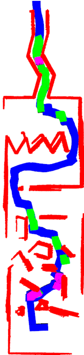
Figure A.83: The path for operator 7 with configuration 6 in the user study. Red is obstacles detected by sensor, blue is the UAV, green is when haptic feedback is activated, and pink indicates collision.
