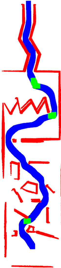
Figure A.49: The path for operator 5 with configuration 1 in the user study. Red is obstacles detected by sensor, blue is the UAV, and green is when haptic feedback is activated.
