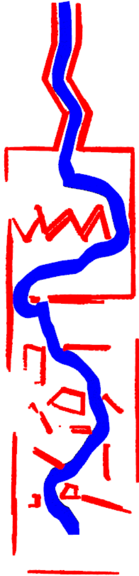
Figure A.53: The path for operator 5 with configuration 3 in the user study. Red is obstacles detected by sensor and blue is the UAV.
