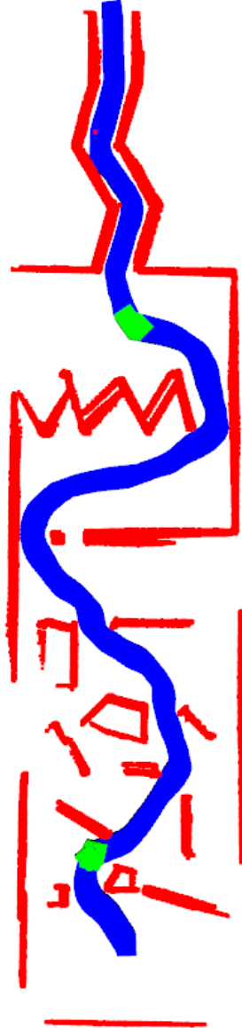
Figure A.57: The path for operator 5 with configuration 5 in the user study. Red is obstacles detected by sensor, blue is the UAV, and green is when haptic feedback is activated.
