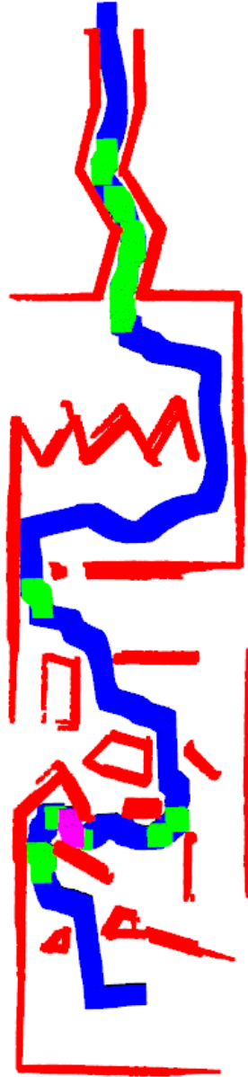
Figure A.47: The path for operator 4 with configuration 6 in the user study. Red is obstacles detected by sensor, blue is the UAV, green is when haptic feedback is activated, and pink indicates collision.
