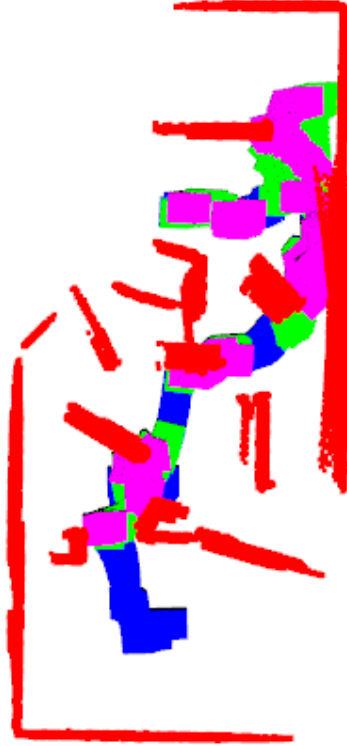
Figure A.39: The path for operator 4 with configuration 2 in the user study. Red is obstacles detected by sensor, blue is the UAV, green is when haptic feedback is activated, and pink indicates collision.
