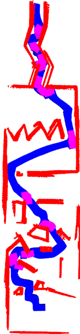
Figure A.19: The path for operator 2 with configuration 4 in the user study. Red is obstacles detected by sensor, blue is the UAV, and pink indicates collision.
