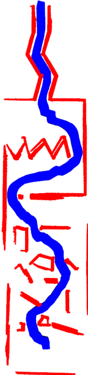
Figure A.29: The path for operator 3 with configuration 3 in the user study. Red is obstacles detected by sensor and blue is the UAV.
