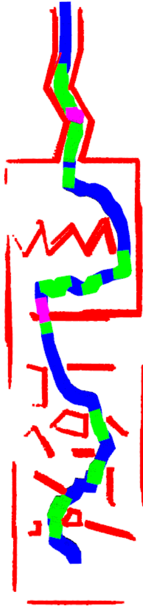
Figure A.35: The path for operator 3 with configuration 6 in the user study. Red is obstacles detected by sensor, blue is the UAV, green is when haptic feedback is activated, and pink indicates collision.
