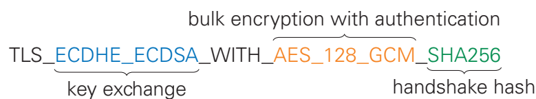
Figure 3.9: The only supported cipher suite by this design. The selected algorithms combine resource efficiency and short computation times.
