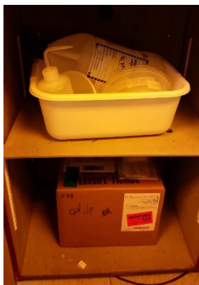
Figure 57. Materials inside the ACID cabinet, with the secondary container containing the three plastic containers (on the top) and the box containing the plastic bottles of Hydrofluoric Acid (1%) (on the bottom).
