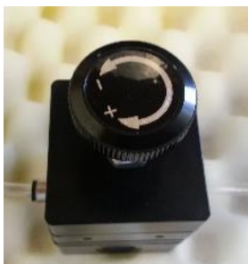
Figure 82. Manual pressure regulator knob with + indicating the direction in which to turn in order to increase the output pressure, and – to decrease the output pressure.
