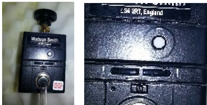
Figure 77. Manual pressure regulator (left) with the white circular dot indicating which side the air should go into (right).
