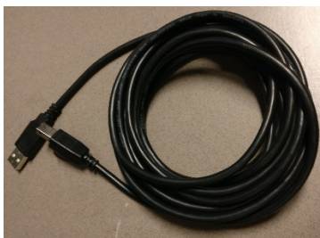
Figure 108. USB type “A to B” cable used to connect the computer to the DAQ module.
