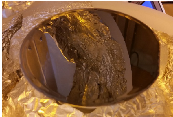
Figure 28. The wafer was placed in a spin coater to obtain a level surface of SU-8 polymer. The spin coater spins the wafer at a certain angular velocity to obtain a desired polymer thickness.
