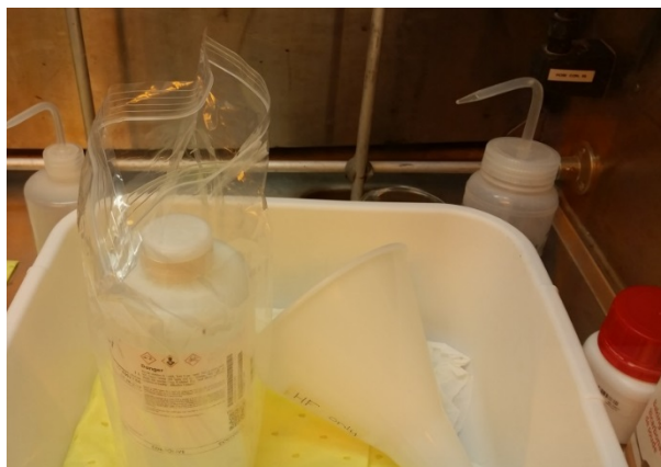
Figure 65. Hydrofluoric Acid (1%) container inside plastic bag, sitting within the secondary plastic container.
