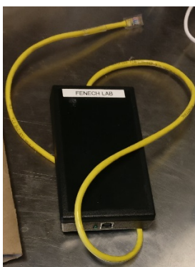
Figure 107. DAQ module with the communication cable already connected.
