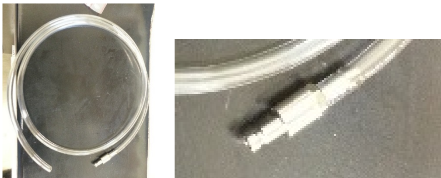
Figure 78. 6 mm × 4 mm (O.D. × I.D.) flexible tubing (left) with the MFCS-EZ metal adapter connected at one end (right).
