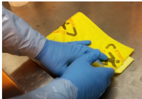
Figure 70. Folding the absorbent sheets to place in the HF chemical solid waste container.
