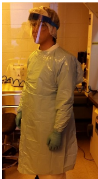
Figure 64. Fully gowned researcher with all personal protective equipment, who is ready to use HF acid.
