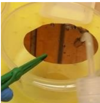
Figure 66. Beading up of DI water on the surface of the processed silicon wafer.
