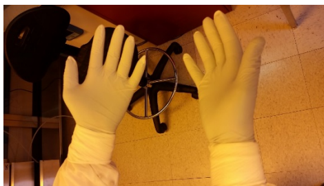
Figure 60. A set of disposable long nitrile clean room gloves goes over the clean room frock and disposable clean room lab coat sleeve cuffs.
