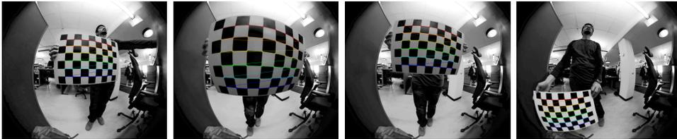
Figure 5.3: Calibration With Checkerboard Pattern.
