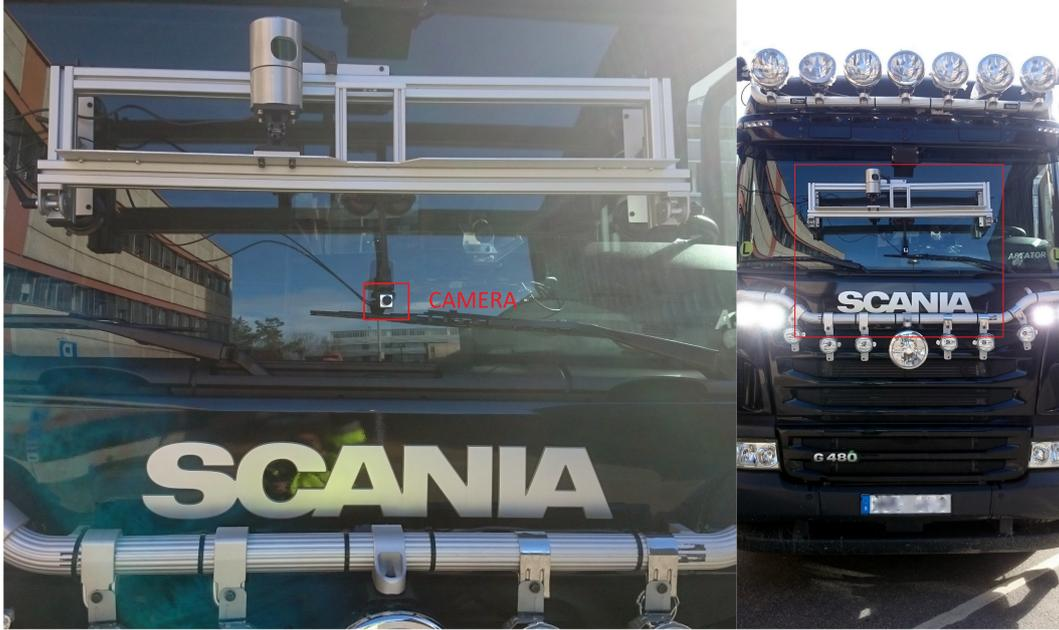
Figure 5.1: Camera placement on the truck.
