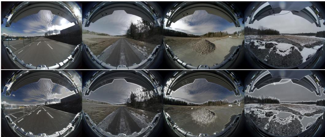
Figure 6.2: Conditions when Gabor filter performed well. (Top) Original and (Bottom) Gabor responses. (L to R) Asphalt road classification, Gravel and mud classification, Gravel pile classification, Mud and snow classification.
