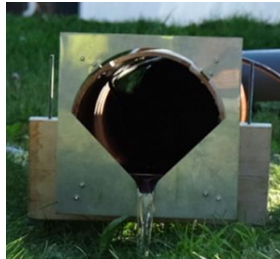
Figure 10 90-degree V-notch weir attached to a pipe channel from experiments in 2015 for inflow measurements.
