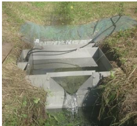
Figure 9 Stainless steel weir box with 90 -degree V-notch weir attached.
