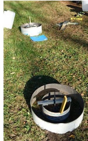
Figure 13 Double-ring infiltrometer tests conducted every 3 m in the swale channel (n=9).
