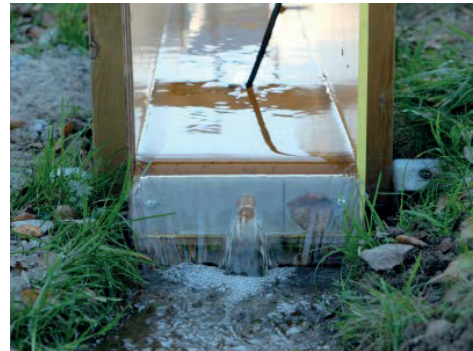
Figure 3: Outlet measurement channel with a compound constriction flow meter (an orifice and a rectangular weir).
