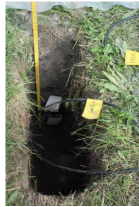
Figure 16 Installation of two WCR-probes for soil water content measurements at 0.3 and 0.6 m depth below the swale channel bottom.
