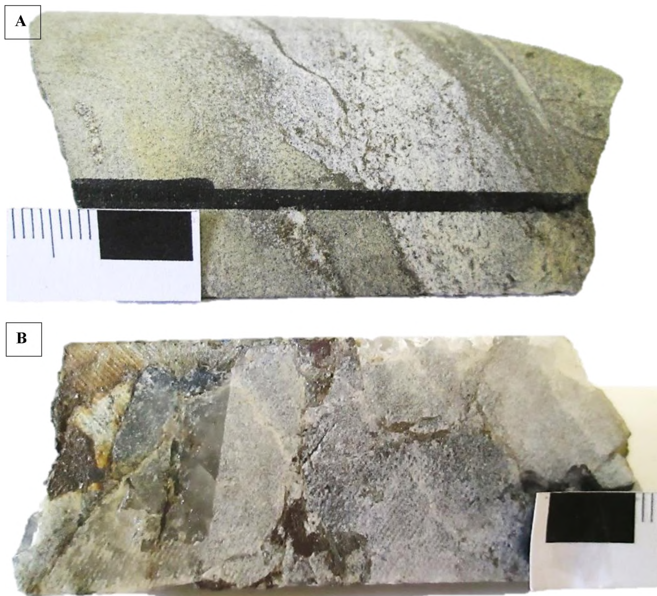
Figure 4.4: Hand specimen photographs of vein samples from Kamituga. A) Sample K17 displaying a quartz vein with biotite-rich marginal zone. B) Sample KG-SIS-1 is a massive quartz vein with arsenopyrite and pyrrhotite grains 1 mm or less in size. Scale is segmented in 1 cm units.
