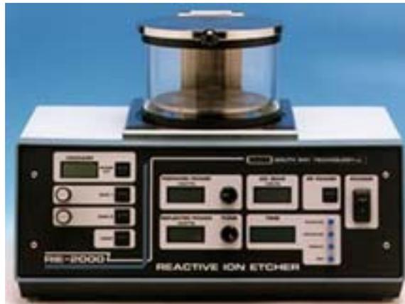
**Figure 6.16: South Bay Technologies RIE-2000 reactive ion etcher.**
