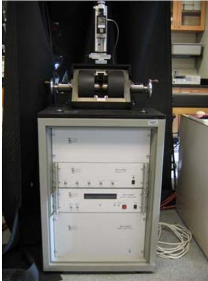
**Figure B1: Picture of the MicroMag AGM.**
