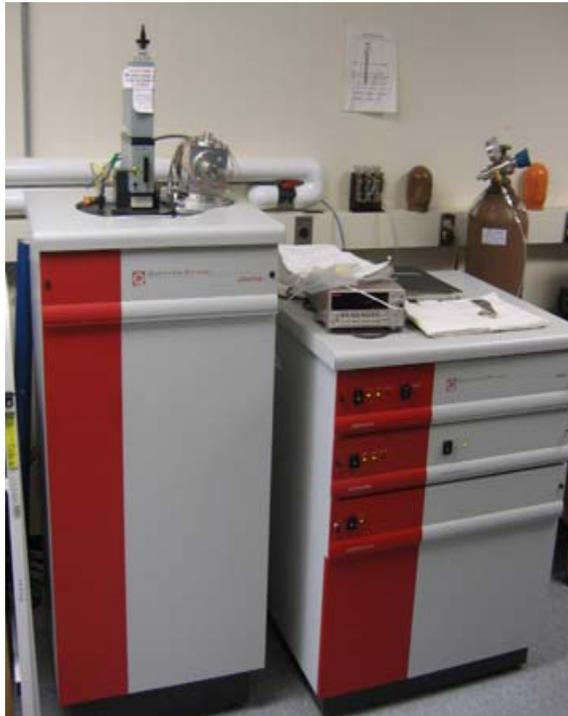
**Figure A1: The Quantum Designs MPMS SQUID. The left box is the SQUID and the right box is the controller unit.**
