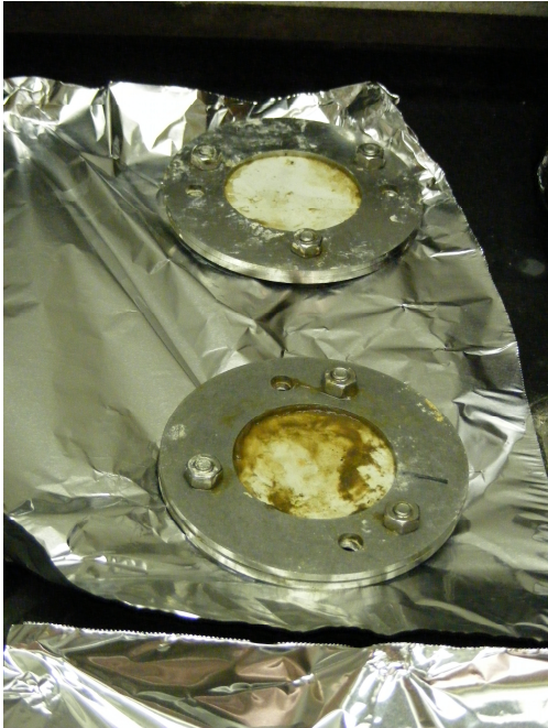
Figure 4-3. POCIS disks after deployment in sewer lines for one month and initial external cleaning.
