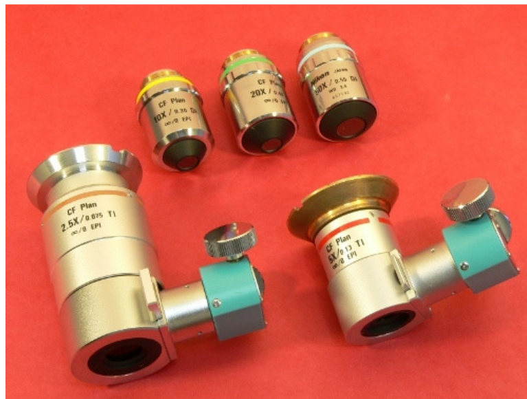
Fig. 8. Interferometric microscope objectives.
