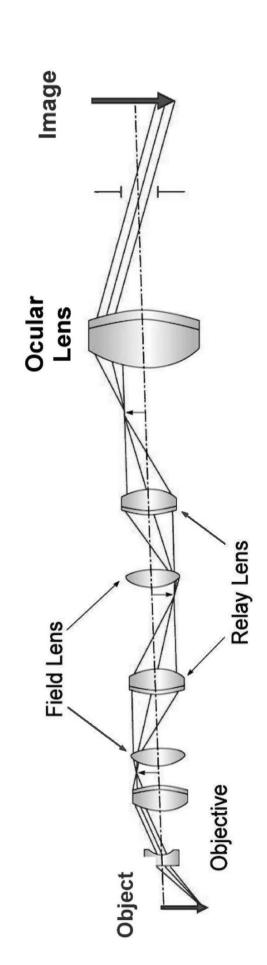
Figure 3-5. Relay lenses in rigid endoscope.
