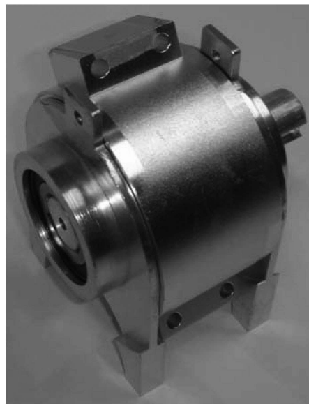
Figure 2.5-1 Fabricated MR actuator (disassembled and assembled)
