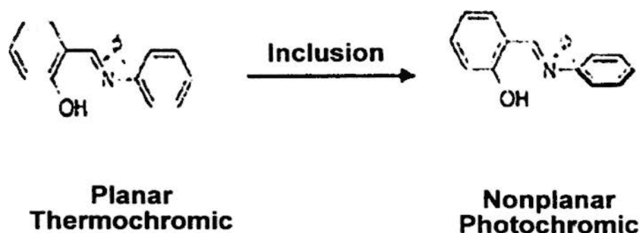
Scheme 1.1.5 Thermo-to-photo-switching of salicylideneanilines by inclusion.
