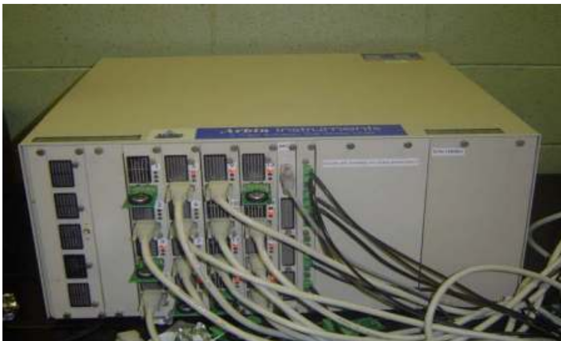
Figure 3.3: 16-Channel BT2000 Battery Testing System
