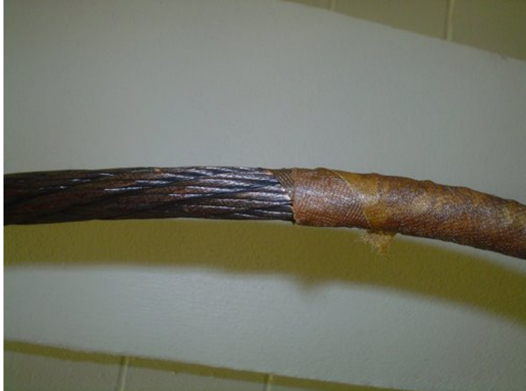
Fig. 79. CT1 dissection after 150,000 ageing hours - Primary Winding
