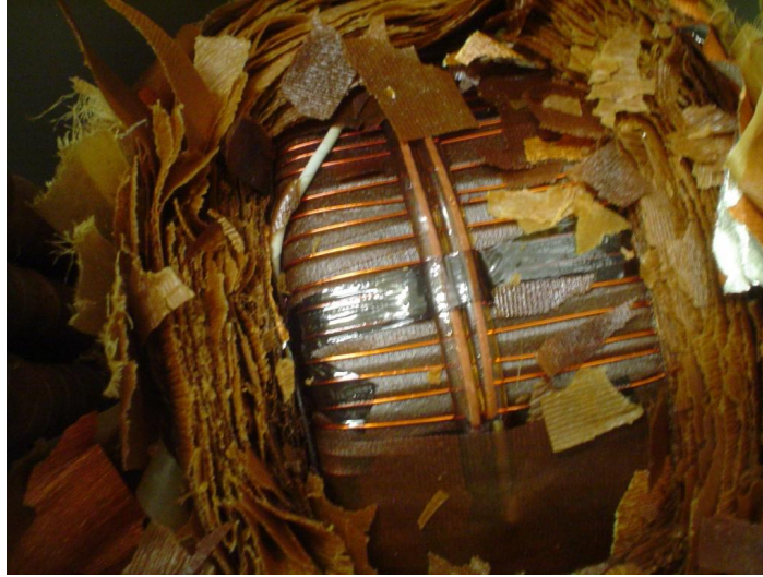
Fig. 77. CT1 Dissection – Temperature Sensors
