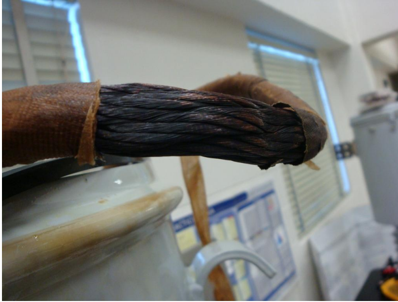
Fig. 117. CT3 dissection after 300,000 ageing hours - Primary Winding
