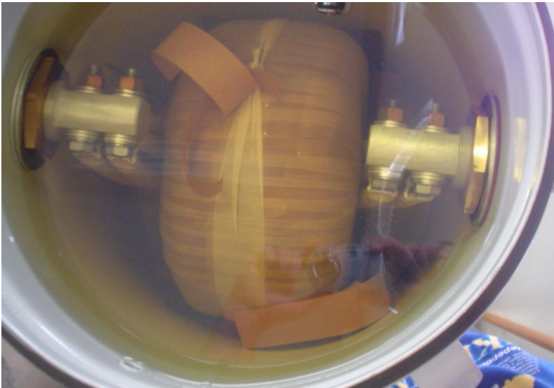
Fig. 36. Paper samples located on the top surface of the core/2-ry winding insulation of CT1
