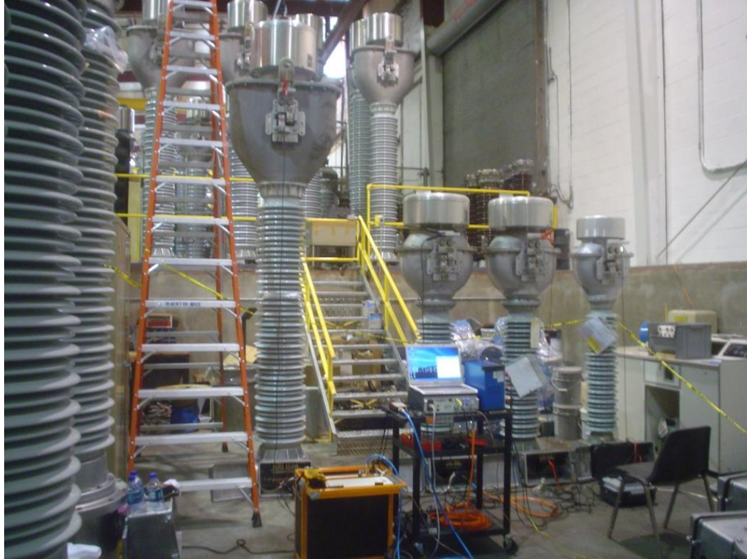
Fig. 159. Dielectric Spectroscopy in the Frequency Domain using IDAX 206 and IDAX 300 on Oil-Immersed Current Transformers at AREVA T&D manufacturing facilities
