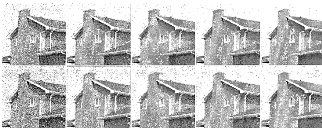
Figure 4.5: Results of the four algorithms on the “House” image with the noise \sigma = 20 (the first row) and \sigma = 30 (the second row). From left to right: the noisy image, the results of GF, BF, NL, and our algorithm.
