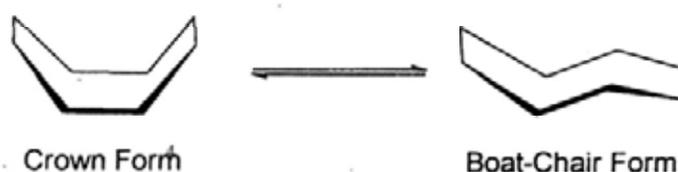
Figure 4.1 Crown Form and Boat-Chair Form of *c*-Octane (Hydrogen Hidden)
