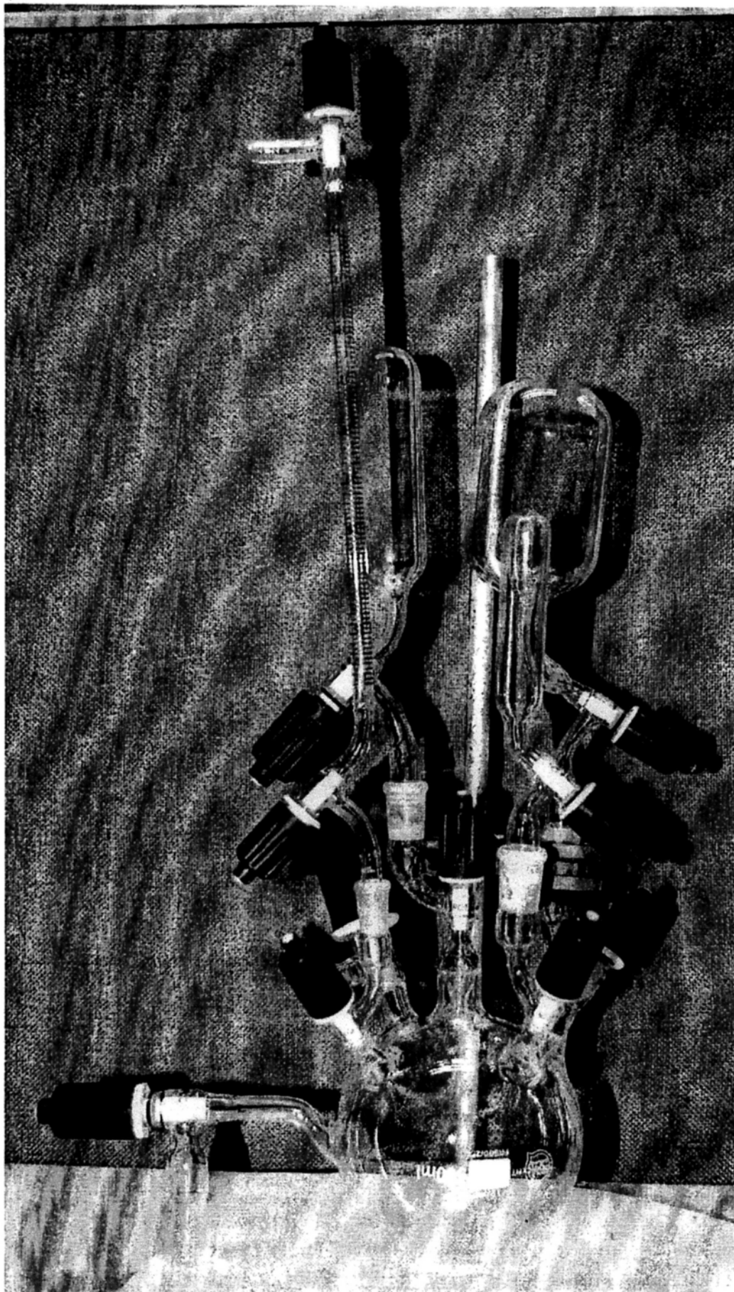
Figure 3.5 Assembled apparatus of home made high vacuum system.
