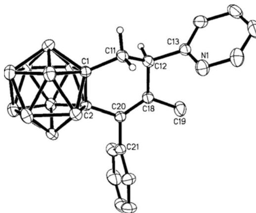
**Figure 4.1.** Molecular structure of **IV-1d**. Selected bond lengths (Å) and angles (deg): C1-C2 1.640(2), C1-C11 1.519 (2), C11-C12 1.536(2), C12-C18 1.531(2), C18-C20 1.340(2), C2-C20 1.503(2), C2-C1-C11 115.8(1), C1-C11-C12 114.4(1), C11-C12-C18 112.8(1), C12-C18-C20 122.6(1), C18-C20-C2 122.2(1), C20-C2-C1 115.9(1).
