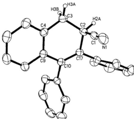
**Figure 4.3.** Molecular structure of **IV-5e**. Selected bond lengths (Å) and angles (deg): C4-C9 1.401(3), C4-C3 1.500 (3), C3-C2 1.524(3), C2-C17 1.537(2), C17-C10 1.342(2), C10-C9 1.476(3), C9-C4-C3 118.2(2), C4-C3-C2 112.1(2), C3-C2-C17 111.5(2), C2-C17-C10 119.3(2), C17-C10-C9 121.3(2), C10-C9-C4 119.7(2).
