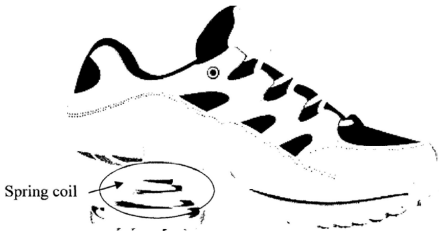
Fig.6-2: The Z-Coil ® footwear with a spring coil attached to the shoe heel, specifically to buffer foot strike and to relieve foot pain [65]
