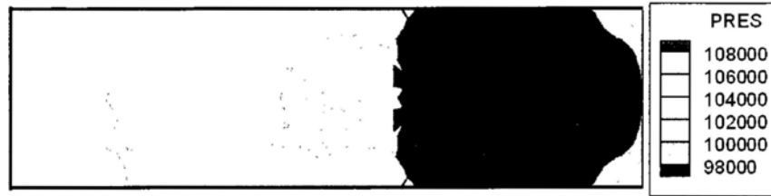
Figure 4.8: Pressure distribution in the micro channel
