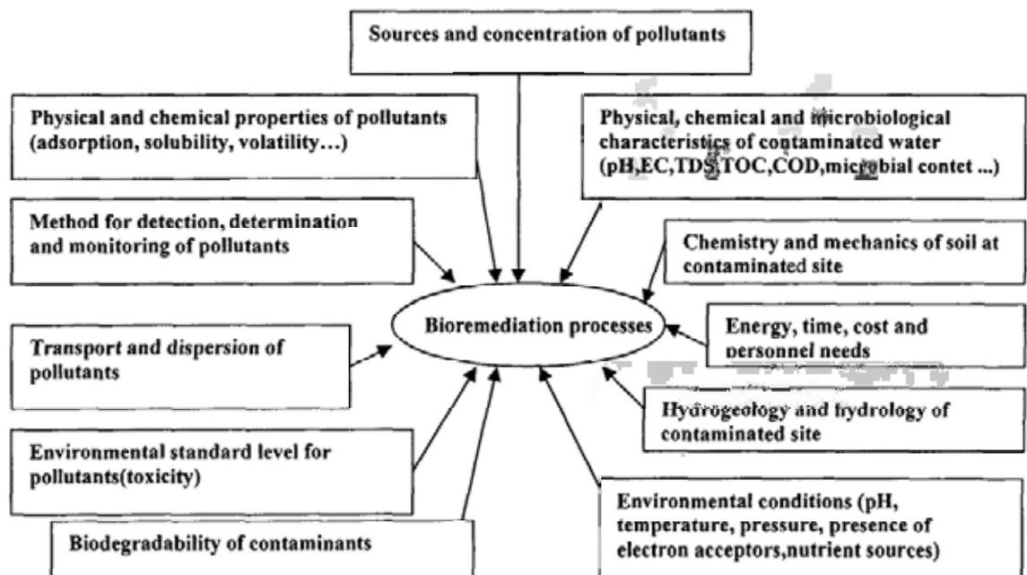
Figure 4.3 Important factors that have to be taken into account to establish an *in-situ* water bioremediation process. (Krishna, 2008)
