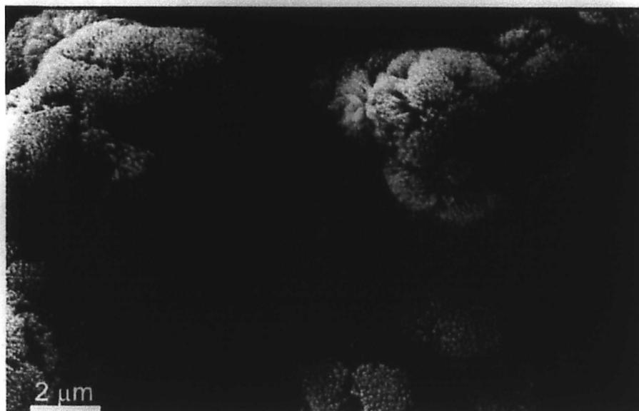
**Figure 7.1** SEM image of the self-assembled rutile TiO<sub>2</sub> by microwave heating TiCl<sub>3</sub> at 200 °C for 1 min.
