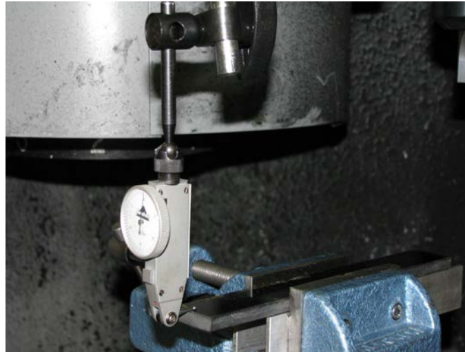
Figure 5-5. Controlling top of workpiece using dial indicator
