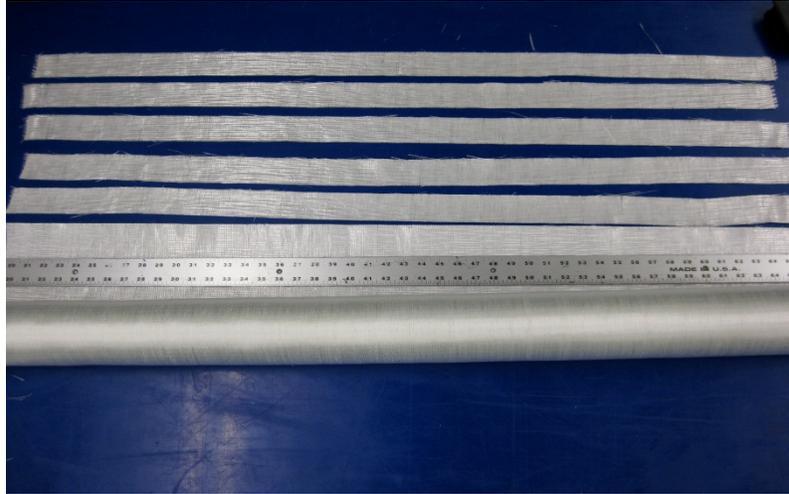
Figure 34. UD Glass fabric cut in 50.4 mm width strips to roll into samples with the desired tows.
