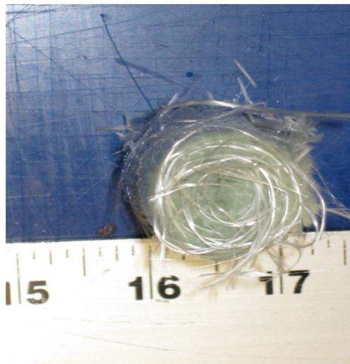
Figure 35. UD Glass fiber strips rolled into 29 mm diameter sample for measurement in the Impedance tube
