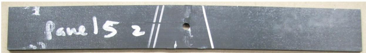
Figure 63. Compressive failure mode for OHC specimen cured at 160°C for 180 min.
