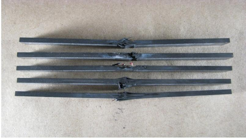
Figure 54. Compressive failure mode for CLC specimens cured at 160°C for 400 min.
