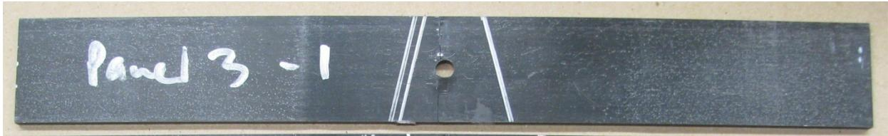
Figure 61. Compressive failure mode for OHC specimen cured at 177°C for 180 min.
