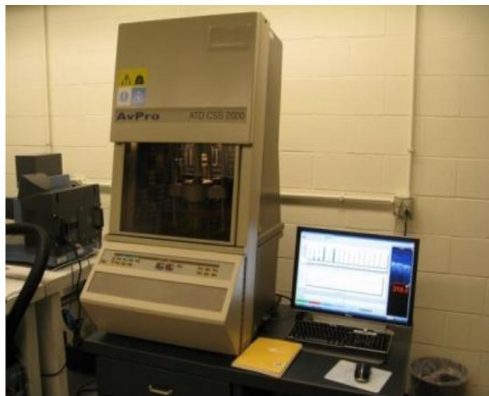
Figure 22. ATD CSS 2000 rheometer.
