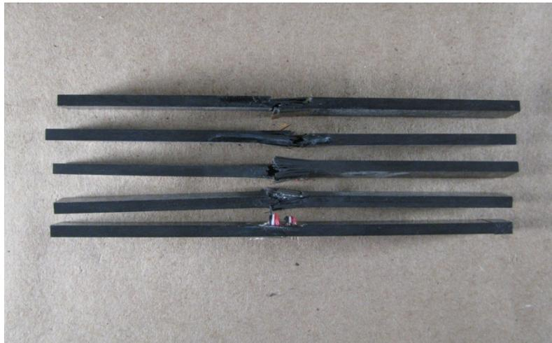
Figure 49. Compressive failure mode for CLC specimens cured at 182°C for 180 min.
