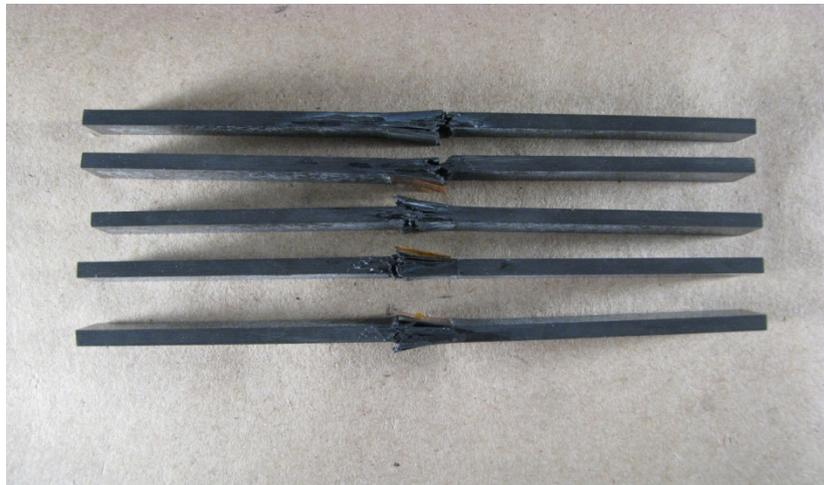
Figure 52. Compressive failure mode for CLC specimens cured at 160°C for 180 min.
