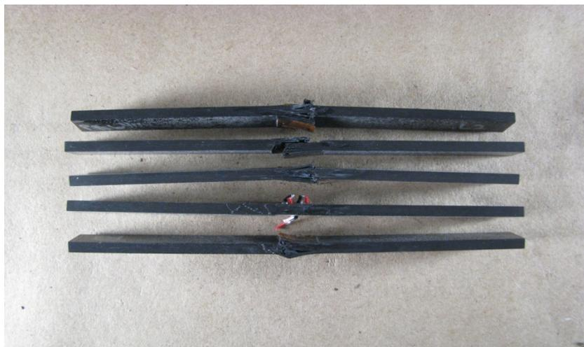
Figure 53. Compressive failure mode for CLC specimens cured at 149°C for 180 min.
