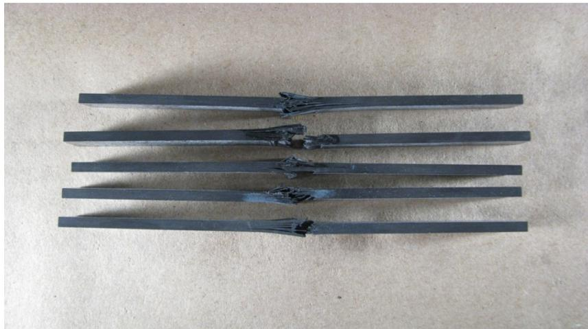
Figure 50. Compressive failure mode for CLC specimens cured at 177°C for 180 min.
