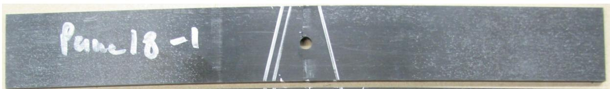
Figure 66. Compressive failure mode for OHC specimen cured at 149°C for 400 min.
