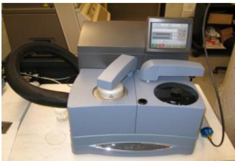
Figure 23. TA Instruments Q2000 differential scanning calorimeter.
