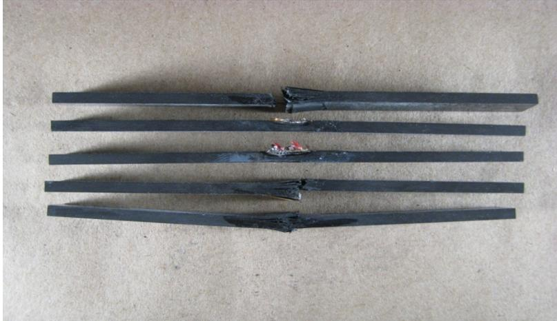
Figure 51. Compressive failure mode for CLC specimens cured at 171°C for 180 min.
