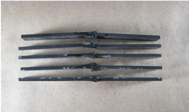
Figure 55. Compressive failure mode for CLC specimens cured at 149°C for 400 min.
