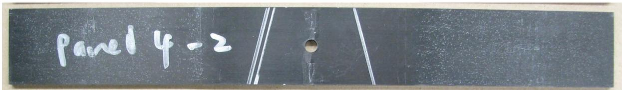
Figure 62. Compressive failure mode for OHC specimen cured at 171°C for 180 min.
