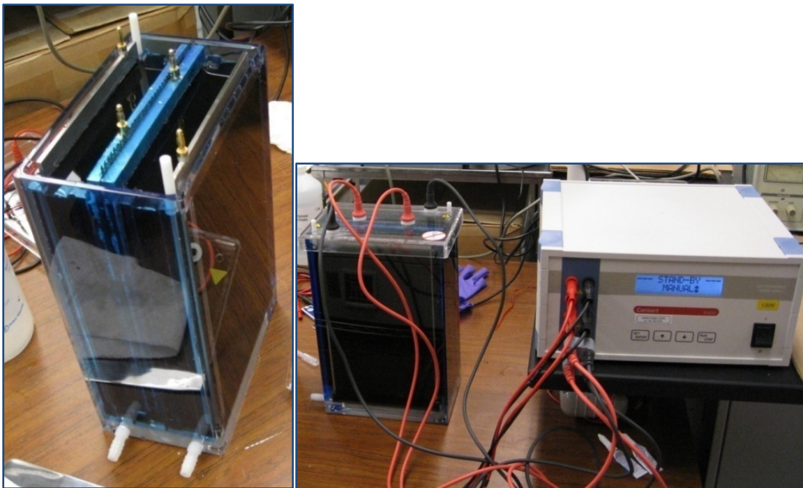
Figure 28. Images of EPD setup before deposition of functionalized carbon nanoparticles.
