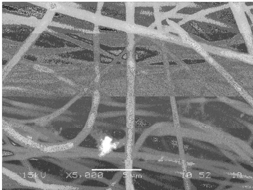
Figure 3-16. SEM image of PAN fibers produced with processing parameters: PAN and DMF (90:10), 1% MWCNTs, v = 25 kv, d = 25 cm, and m = 1 ml/hr.
