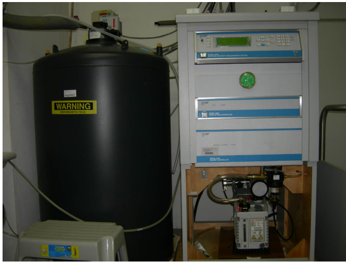
FIGURE A.4: Physical property measurement system from Quantum Design, capable of measuring DC resistivity or electro-transport, magnetometry (for example, AC susceptibility), thermal transport, and heat capacity.
