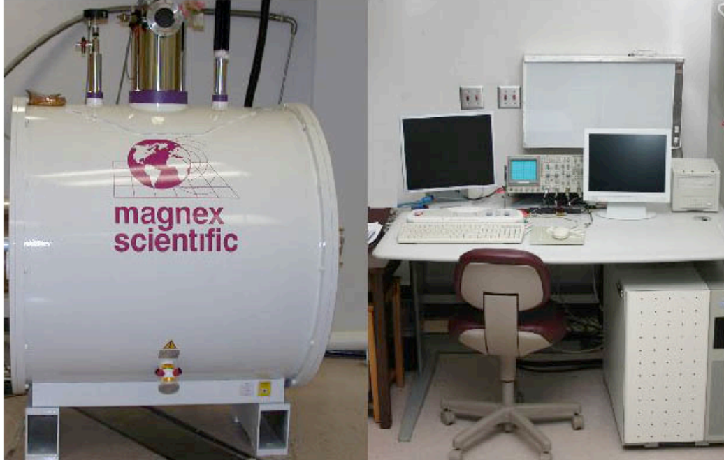
Figure 4: 7T magnet with GE EPIC console
