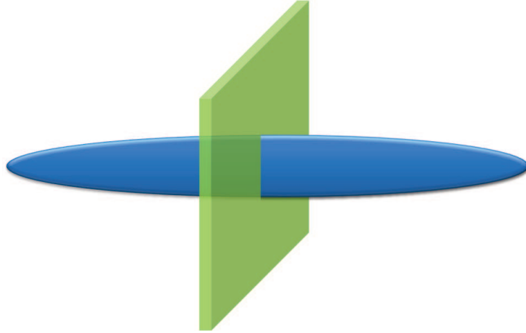
Figure 5.3: A sheet potential of green light incident on the axial center of the trapped atoms
