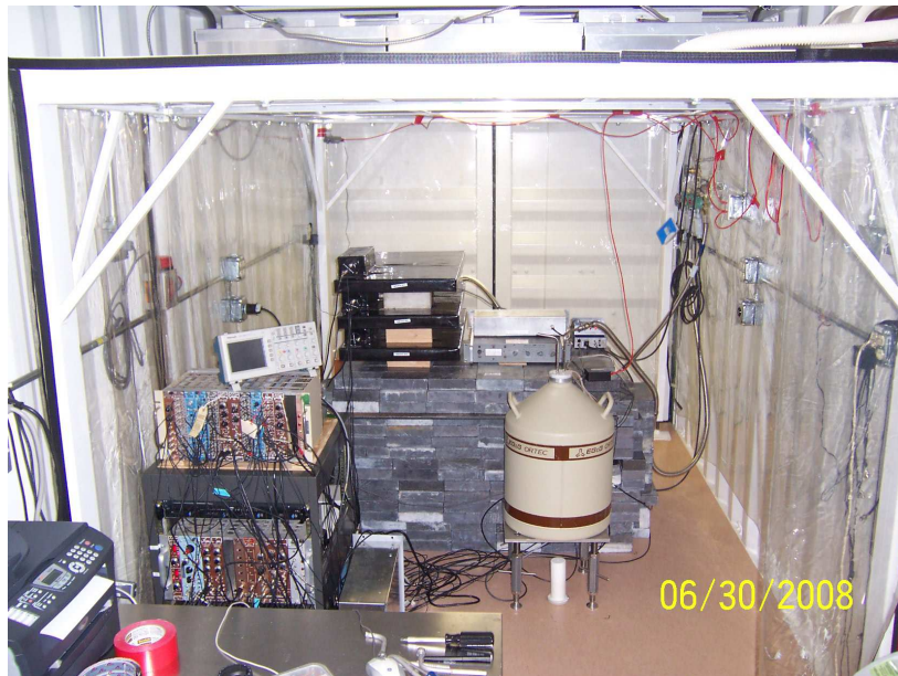
FIGURE 3.4: (Color online) A view of the TUNL-ITEP double-beta decay setup from the door of the TUNL connex trailer.
