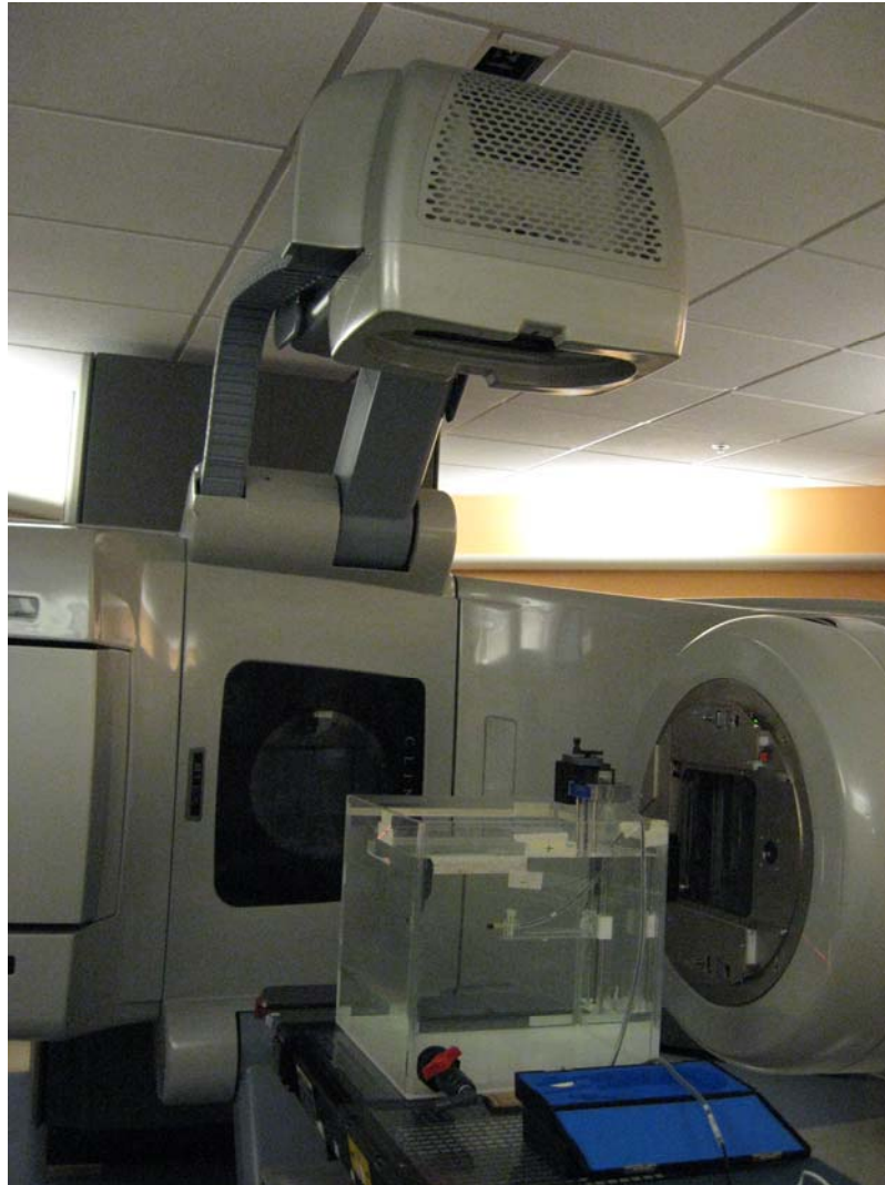
FIG. 2. Lateral and depth dose profile measurement setup with a water tank and an ion chamber.
