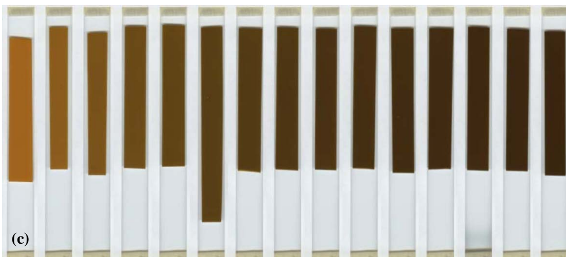
FIG. 17. Results of the radiochromic film calibration. (a) Calibration curve as pixel value vs. exposure, (b) calibration curve as exposure vs. optical density, and (c) raw film images. Note that the x-axis in Fig. 17(b) is on the logarithmic scale ( \log_{10} ). The numbers under the raw film images represent the average exposure values (unit in R).
