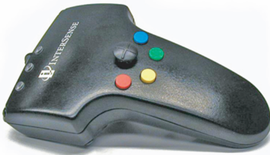
Figure 4-4 - InterSense Ultrasonic 3D Controller
