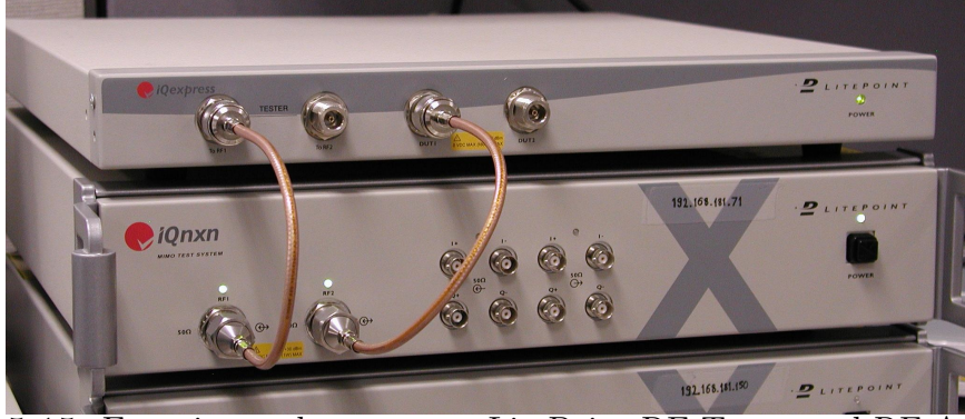
FIGURE 5.15: Experimental test setup, LitePoint RF Tester and RF Attenuator
