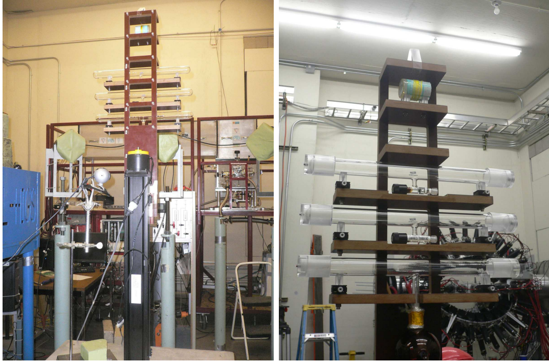
FIGURE 7.2: (Left) The six layer support is attached to the automated motor control. A web camera was set up to monitor the movement of the support to make sure the right target cell was in place. (Right) A close look at the six layer support. From top to bottom: aluminum plate, liquid D_2O target, completely empty/air, D_2 gas target, N_2 gas target and ^3He target. The three lower targets have end caps attached to both ends for initial alignment.
