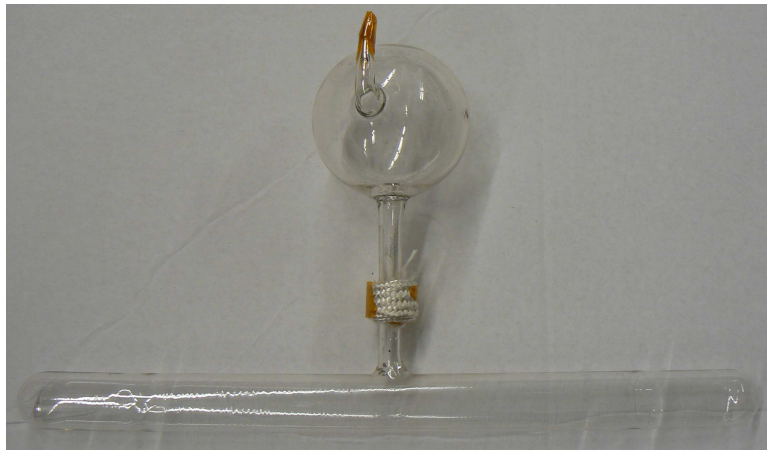
FIGURE 4.3: The ^3\text{He} cell used in the experiment. It is a double-cell system: the upper pumping chamber and lower target chamber. The pumping chamber has a diameter of 9 cm and the target chamber has a diameter of 3 cm, a length of 40 cm. A transfer tube connects the two chambers.
