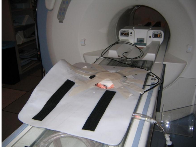
Figure 5.5: Picture of phantom secured inside the breast applicator. Tape was used to secure the phantom inside the applicator and prevent its movement with the volunteer's breathing.
