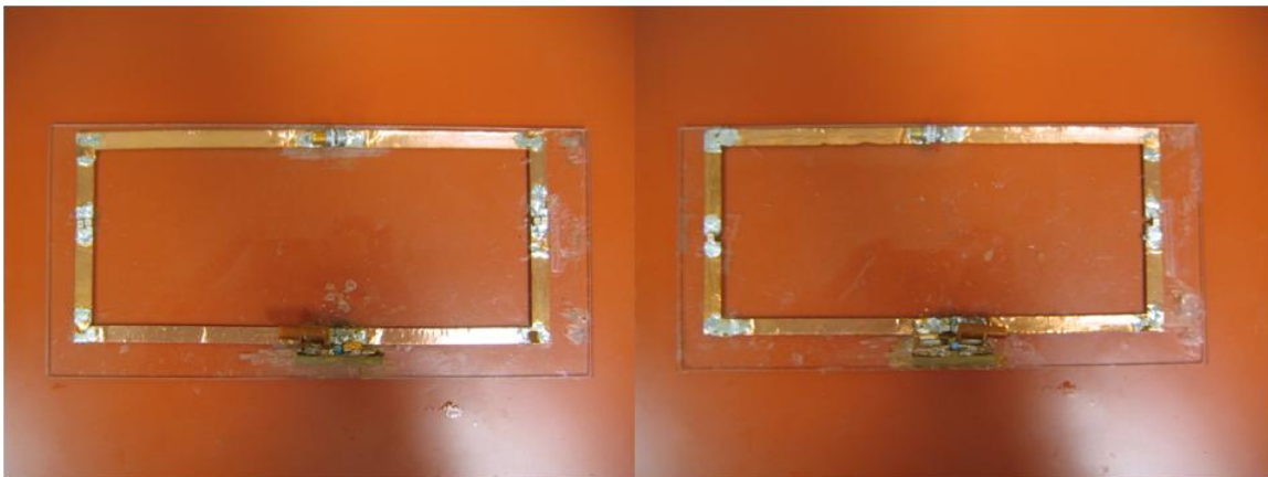
Figure 2.9: Pictures of both prototype local imaging coils
