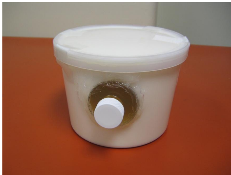
Figure 5.3: Picture of the fat-water phantom developed for the breath hold experiments
