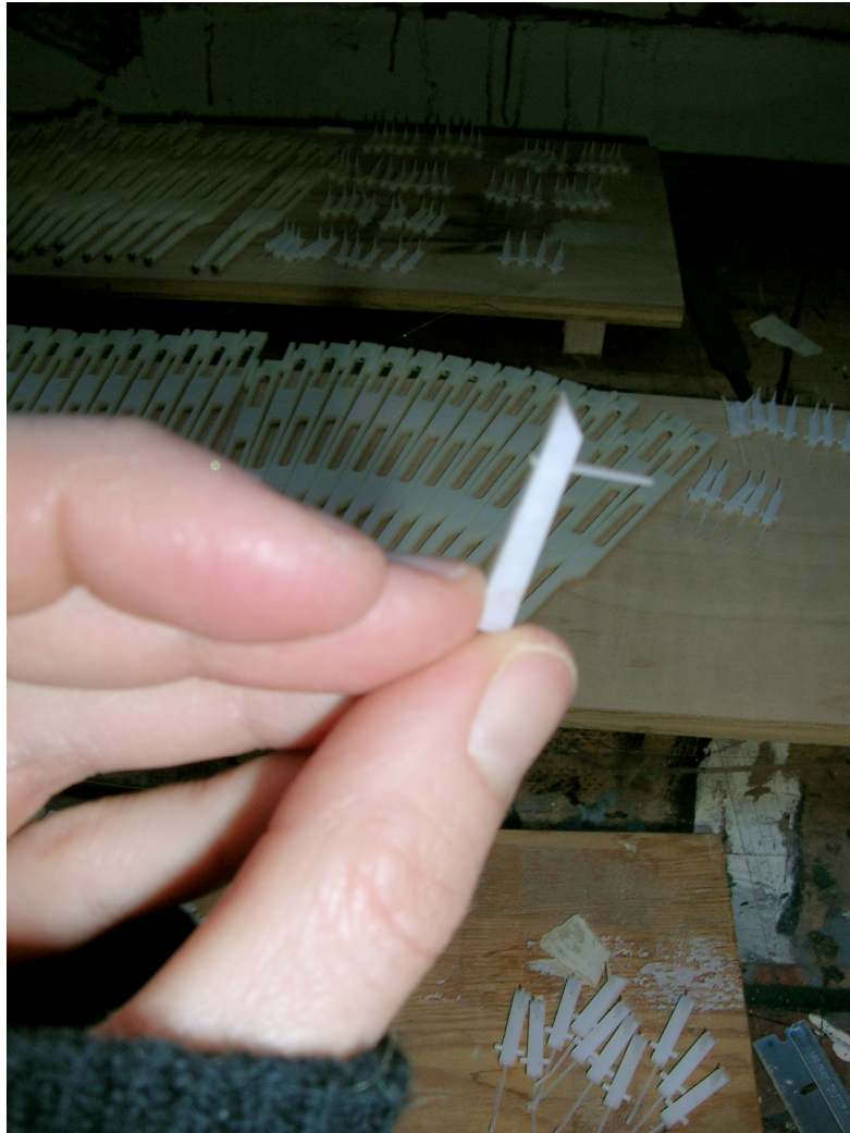
Figure 8: Fitting many plectra into many tongues. Photo by the author.
