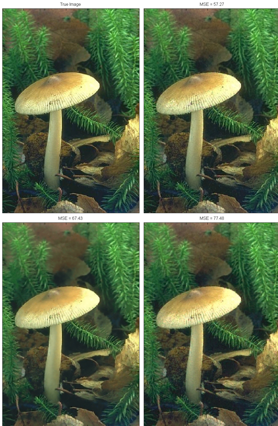
FIGURE 6.7: Reconstruction results for 75% missing for (upper-right) iMMSE, (lower-left) Proposed algorithm, (lower-right) K-SVD.
