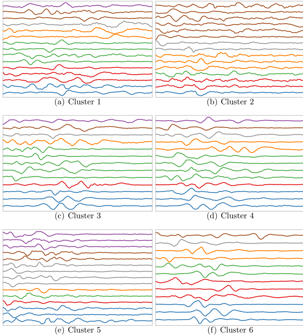
FIGURE 6.5: Determined clustering for landmine A-scans with color depicting different landmine types. Only the 6 clusters containing the most A-scans are shown.
