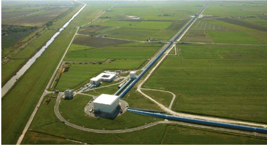
Figure 2.4: Virgo observatory in Cascina, Italy. Each arm measure three kilometres in length ( www.apc.univ-paris7.fr )
