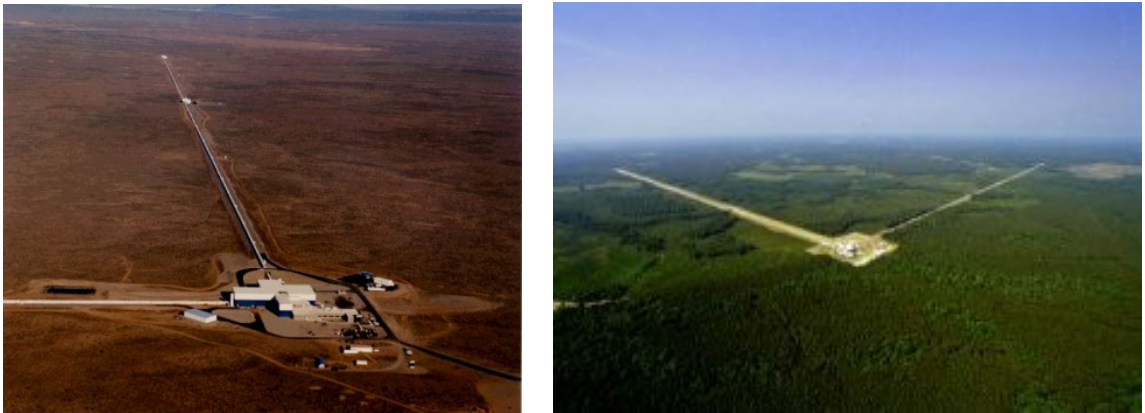
Figure 2.3: The two L-shaped observatories of LIGO, in Hanford, Washington (left) and Livingston, Louisiana (right). The arms are four kilometres in length (astro.berkeley.edu)
