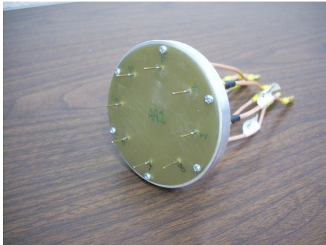
Figure 2 8 element UCA on a ground skirt
