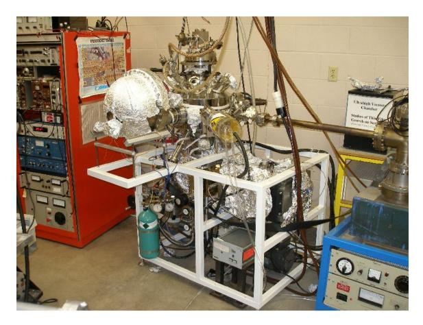
Figure 2.5: New UHV chamber in operation installed on the beam line.
