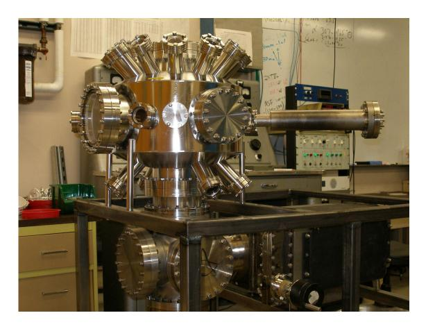
Figure 2.2: Newly constructed UHV chamber mounted on stand before initial vaccum testing.
