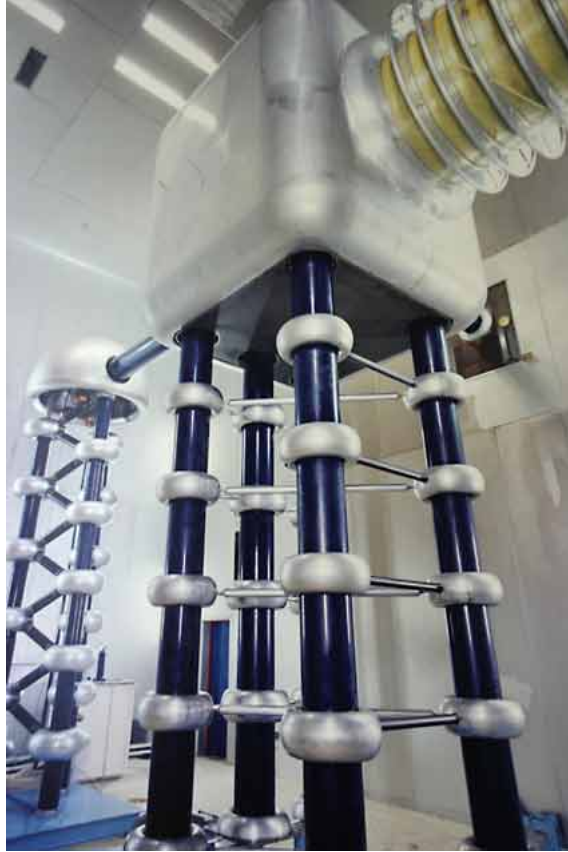
Figure 3.2: Cockcroft-Walton generator at Fermilab.
