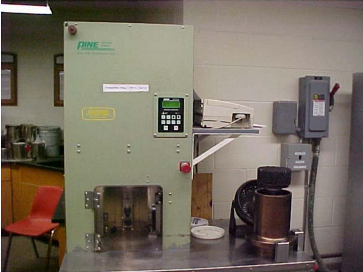
**Figure 3.4 Superpave Gyrotory Compactor**
