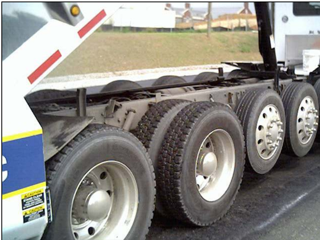
Figure 2.6 Testing trackless tack performance on Virginia road (Trenton, Todd, and Kevin 2010)
