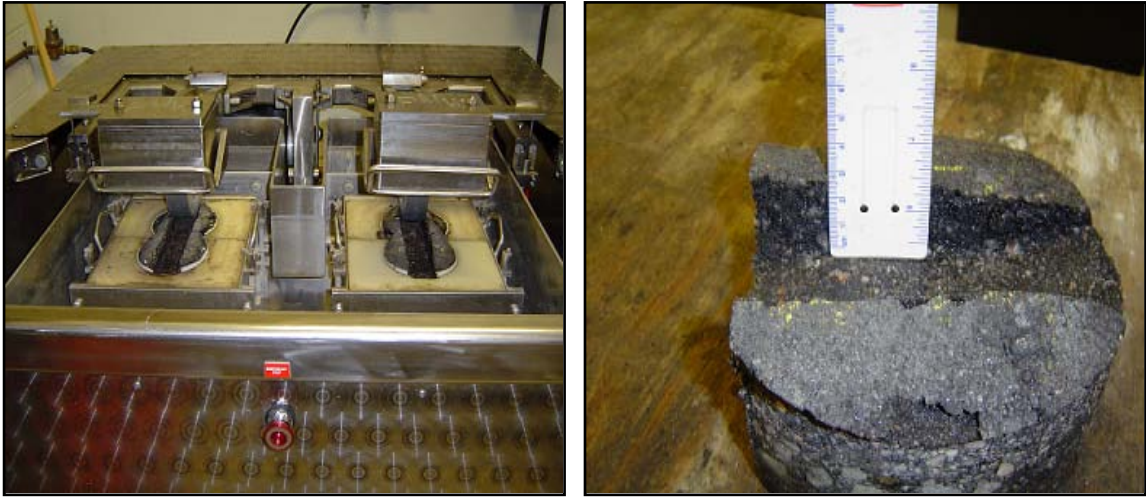
Figure 3.9 Experimental setup and failure surface on field cores
