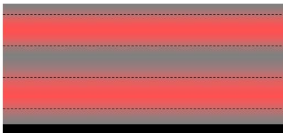
Figure 1.1 Schematic of PE multilayer film. Grey color represents positively charged polymer and red color represents negatively charged polymer. Note the
