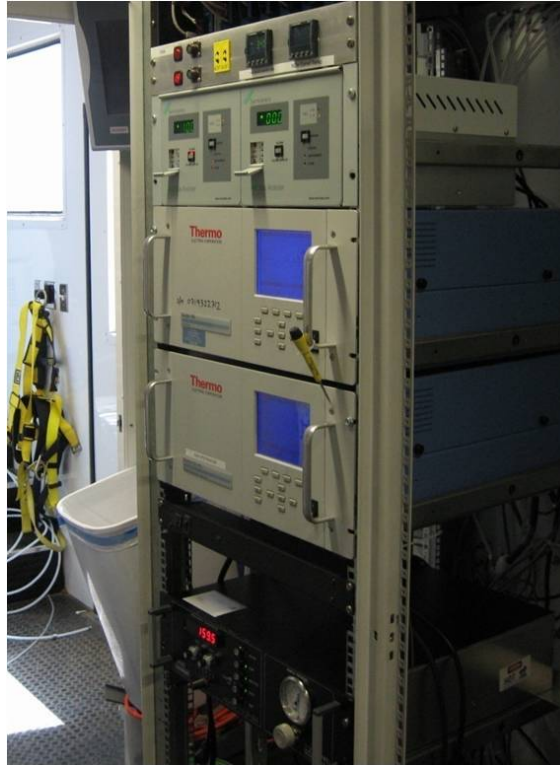
Figure D.3 FTIR analyzer used in Engine 1 mapping
