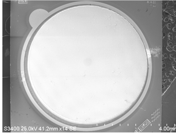
Figure 4.1: Evaporated LiF film coating on a diode structure.
