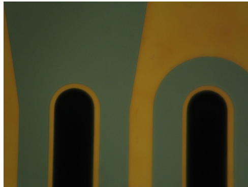
Figure 6.4: Close-up view of the diode array showing the buffer space between the trench (black) and the diffusion layer (blue-green).
