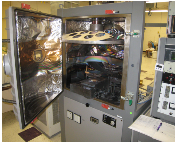
Figure 3.11: Typical evaporation apparatus and geometry. Wafers load into the top of the chamber while the source material rests in a small crucible at the bottom of the chamber.
